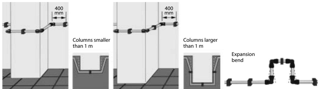
Compressed air pipelines should always incorporate a water separator (swan neck bend).
