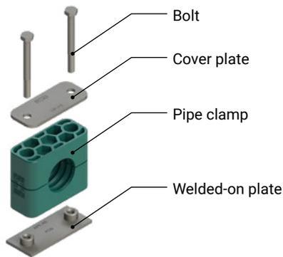
Weld the welded-on plates to a supporting surface strong enough to carry the applied loads. Take the alignment of the clamps into account. Fit the bottom clamp-half onto the welded-on plate, place the pipe into it, fit the second clamp-half and tighten with the bolts. Avoid pre-tensioning the blocks (the clamp halves should not touch after installation)! Do not weld with the plastic clamps in place! Elongated welded-on plates can be attached to the supporting surface with threaded fasteners.
