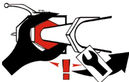
*When tightening fittings (on customer connections), always counterhold using a suitable tool.*
