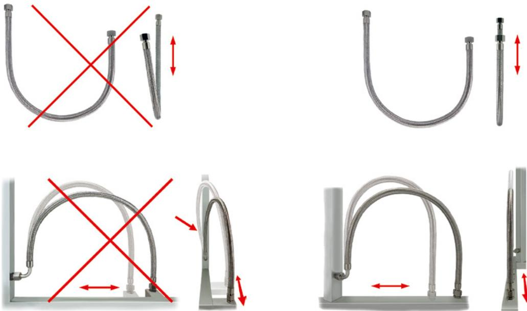
Where movement occurs, the longitudinal axis of the pipeline or hose must be in the same plane as the direction of movement.
