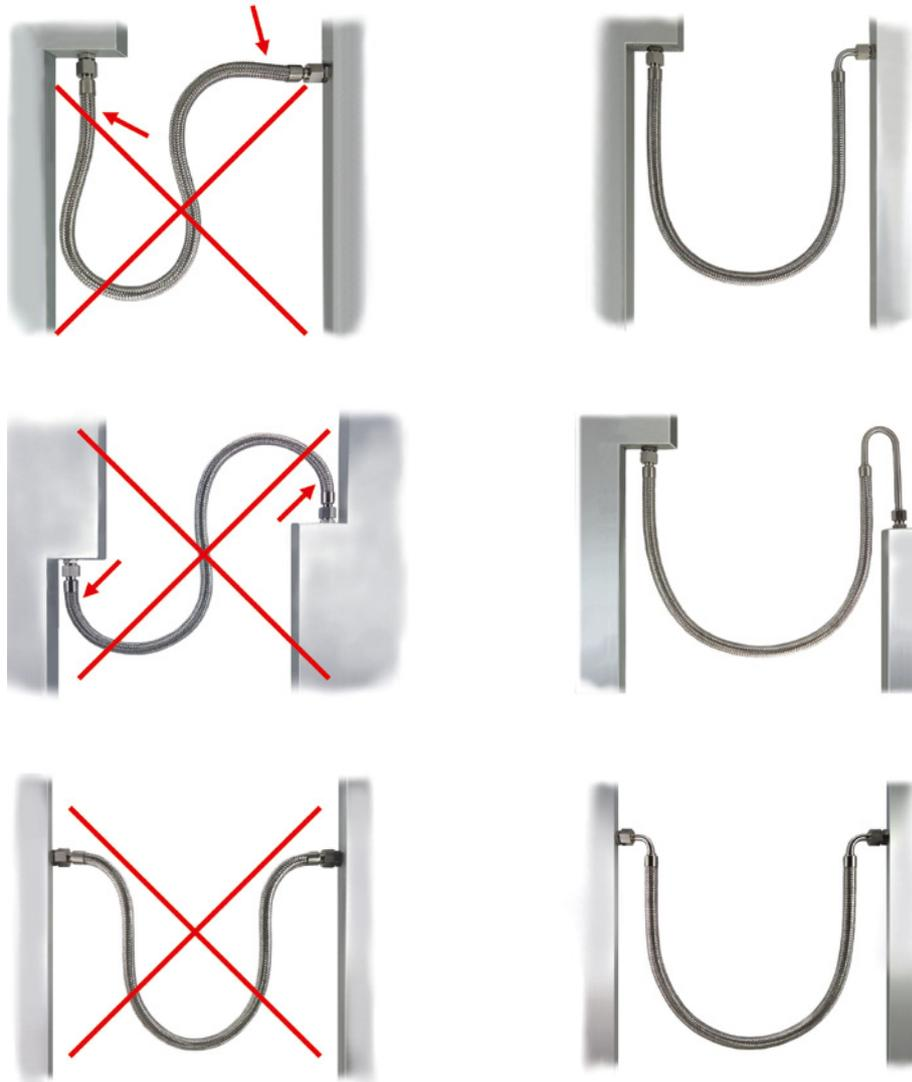
Incorrect installation of a hose line can place high bending loads on the hose close to the connections. This mistake is avoided by installing pipe bends.
