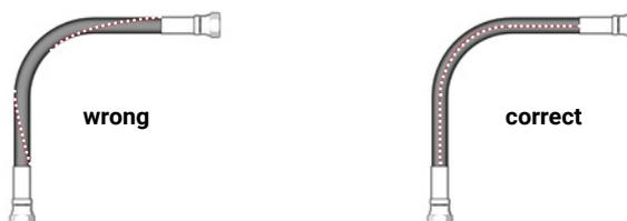
Torsional loads are always to be avoided because they lead to early failure of the hose line. They can occur due to incorrect installation.
