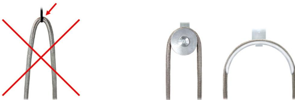
Laying the hose line over a saddle or a roller of the appropriate diameter prevents the hose line from kinking.
