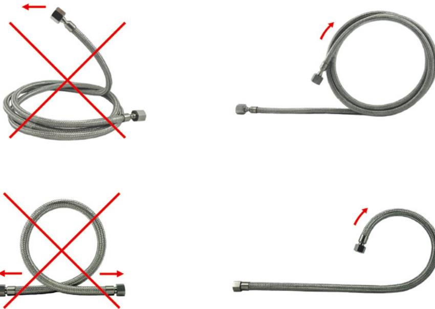
Pulling on the ends of an uncoiled hose line may twist it and cause damaging torsional loads. Observe the smallest allowable bending radius. This mistake is avoided by coiling and uncoiling correctly.
