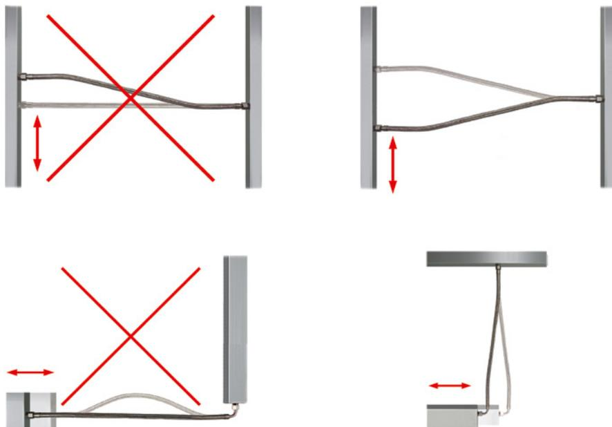
Install at right angles to the expansion direction, preconfigure for half of the occurring expansion, avoid specifying too short a length otherwise the hose will be subject to tension in the full expansion position.
