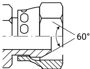
The counterpart is the HN connection (AGN male), which has a sealing surface in the form of a 60° inner cone. The HN connection makes a metallic seal in combination with an AN connection.
