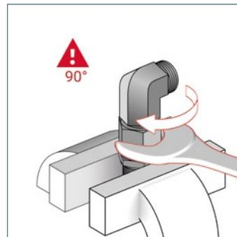
In order to ensure correct installation, the recommended minimum torques should not be exceeded by more than 10 % during assembly.
