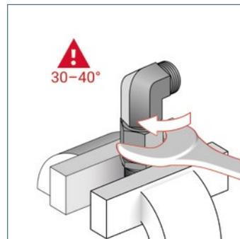
In order to ensure correct installation, the recommended minimum torques should not be exceeded by more than 30 % during assembly.
