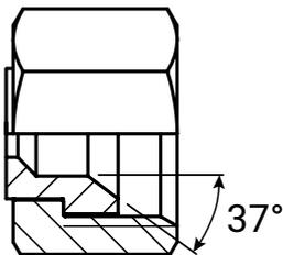
The HJ connection (AGJ) with its sealing surface in the form of a 37° outer cone and the UNF external thread (male) form the counterpart to the AJ connection.
